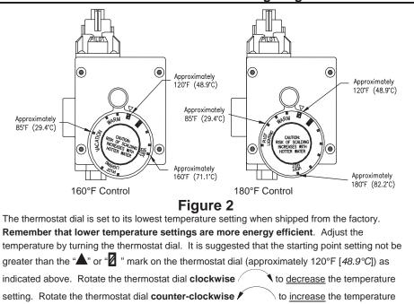
setting. Adjust the dial until the minimum acceptable temperature is achieved (See figure 2 above for approximate temperature settings).
