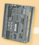
Zone Control Panels are compatible with most conventional, heat pump, and geothermal multi-stage systems. The solid state circuitry incorporates optional features such as: outdoor air temperature sensing, automatic heat/cool changeover, purge cycle and has built in diagnostics.
