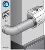
Locate manual or digital humidifier control on the return 6" above the humidifier or bypass duct.
