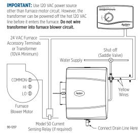
IMPORTANT: When Model 50 current sensing relay is used, wire Model 50 current sensing relay into 24 VAC humidifier control circuit only! Do not install in transformer primary circuit.
