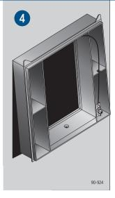
Position base in duct opening top-first so hooks engage sheet metal at top. Insert bottom of base and slide down to engage hooks at bottom.
