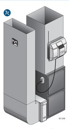
Locate manual or digital humidifier control on the return.
