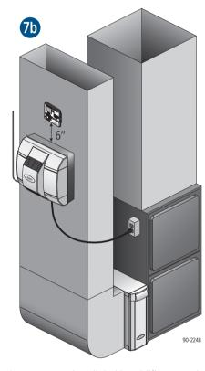
Locate manual or digital humidifier control on the return at least 6" above the humidifier.
