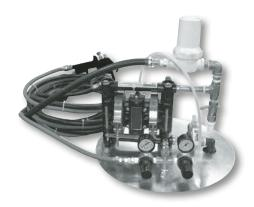
The revamped Universal version of our Super Sprayfast Adhesive Applicator (SSFU) machine makes it possible to use the same applicator on either a 5 gallon bucket or 55 gallon drum. In addition, it now also includes a new flush kit for easy clean up and maintenance. The SSFU features an acetal/teflon diaphragm pump circulating system and surge tank to provide quick, easy and even spray, with minimal overspray.
