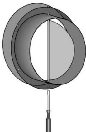
Push and turn with slotted screwdriver. Damper automatically locks when pressure is released.
