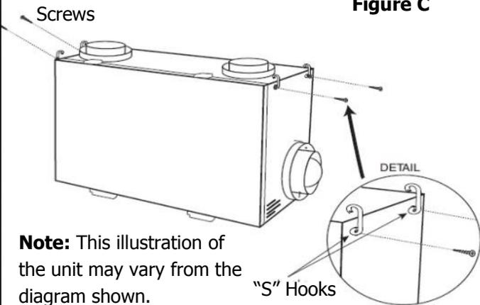
**Step 4:** Level the unit from right to left to right and front to back. Adjust the unit up by pulling down vertically on the hand loops while lifting up on the bottom of the cabinet.
