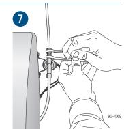
Tighten water line by double wrenching.
