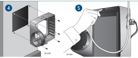
Insert feed tube into distribution tray.
